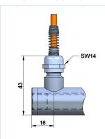
Sensors with cable output have a cable fitting and a spring for bend protection of the cable. For installation, the bending radius should not be less than 3 times the cable diameter. The standard cable length is 2 m.
